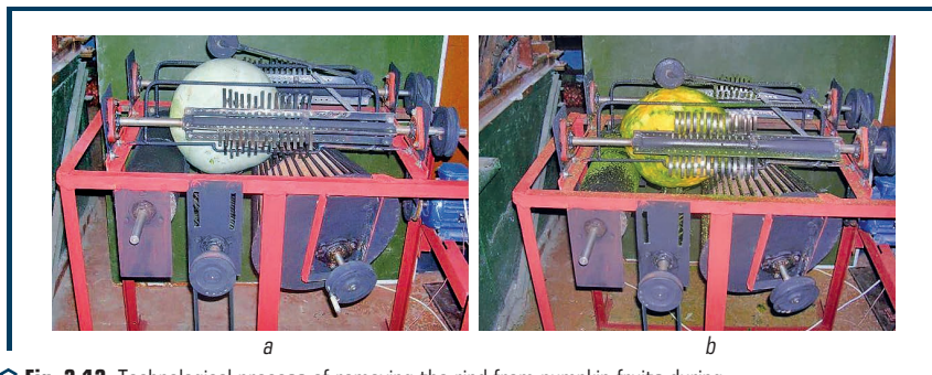
Fig. 3.13 Technological process of removing the rind from pumpkin fruits during a multifactorial experiment: a – the initial state of the fruit; b – type of fruit after peeling
