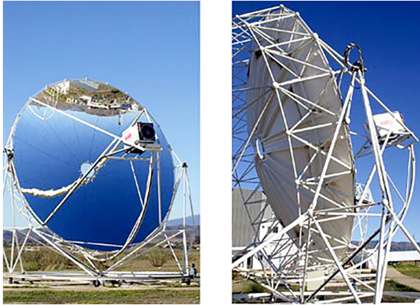
Fig. 2.5 Solar concentrator from EuroDish Source: [29]
